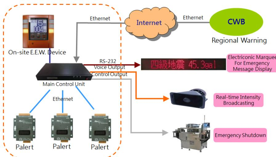
Providing two outputs and supporting the industrial communications standard Modbus TCP/RTU, Palert is an ideal product for seismic safety control in numerous applications.
